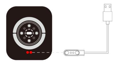
Align the two contacts of the charger to the charging position on the back of the watch and connect the other end to the standard USB interface to charge.
